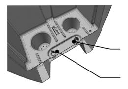
For indoor use, press the red plugs down firmly into the overflow drainage hole to seal the planter before use.
