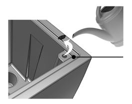
Remove fill port plug for direct access to the water reservoir.
