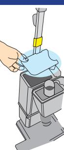
To check motor intake filter, open filter cover and remove Intercept Micro Filter. Confirm that motor intake filter is secure in bottom of filter housing.
