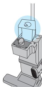
Replace Intercept Micro Filter and close filter cover. If no Intercept Micro Filter is in place the vacuum will not operate.
