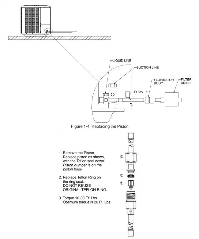
Figure 1-5. Piston Components
