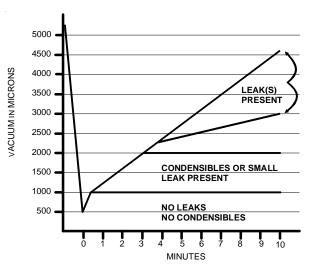
If the pressure rises to 1000 microns or less and remains steady the system is considered leak-free; proceed to startup.
