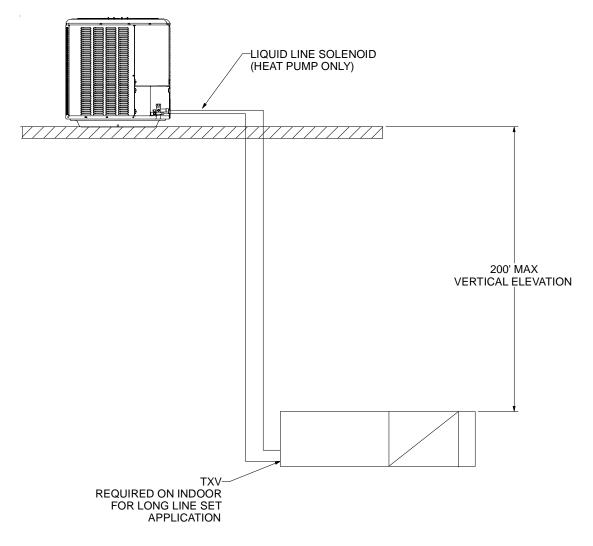
Figure 1-6. Elevation Between Outdoor and Indoor Units
