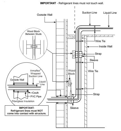
Figure 1-2. Installation of Refrigerant Piping (Vertical)
