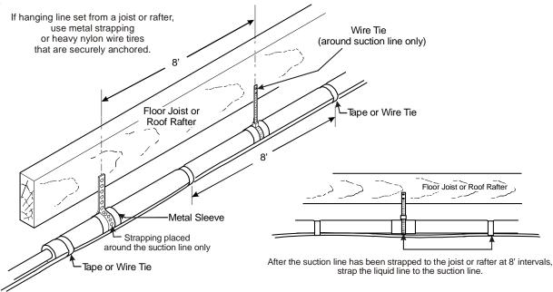
Figure 1-3. Installation of Refrigerant Piping (Horizontal)
